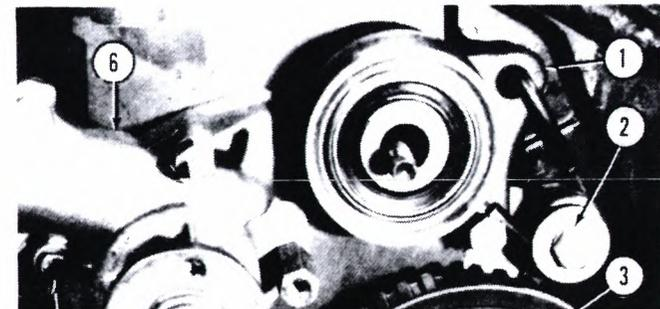
With tensioner bracket bolt (4) slightly loose, pry tensioner pulley (11) to belt-slackened position and tighten tensioner bracket bolt.
