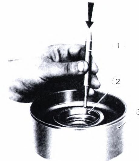
Thoroughly clean drum (3). Install new bushing. Use installer tool 23130-2 and handle 8093. Install bushing flush with rear face of drum hub.
