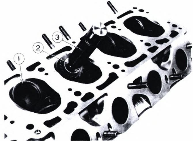
The width of intake and exhaust valve seats, after narrowing should be  $L = 0.08$  inch (2 mm) approximately.
