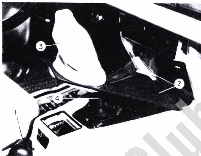
Unclip plastic retainer (1) at bottom of gearshift lever assembly and separate top half (2) of lever from bottom half as shown.
