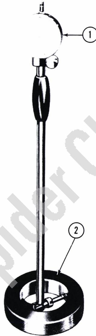
Check cylinder bore at three points both lengthwise and cross-wise.
